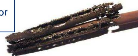
*Effect of the boiling crisis on a heated rod*
